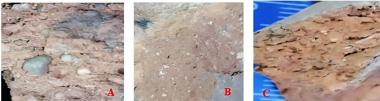
[FIGURE 3]: Stereomicroscope examination. A. First sample (quartz); B. Second sample (calcite); C. Third sample (burnt straw, gaps & cracks) © Done by the researcher
