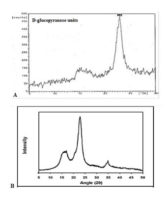
[FIGURE 4]: A- X-ray diffraction pattern of archaeological archive paper (done by researcher) compared to B- the standard X-ray diffraction spectra of cellulose crystallinity<sup>10</sup>
