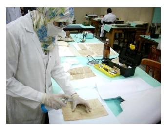
[FIGURE 9]: The disinfection process applied by spray techniques.
