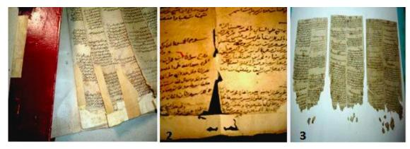
[FIGURE 2]: Visual Assessment of the paper archive showing different aspects of deterioration on the paper sheets: 1- Inappropriate old restoration, some dirty moist dust found on the surface and warping of some parts of edges; 2- Contraction in different places, embrittlement of some parts and loosening in the stitching; 3- The loosening in some parts resulted in separation of small parts from the sheets.
