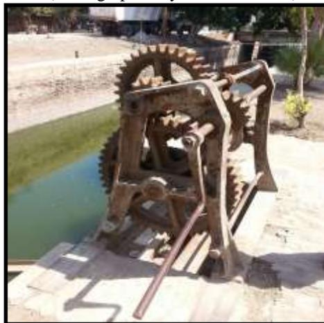
**Plate No. 15:** The crane used in Bagouria Lock.
